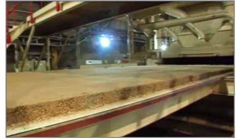
Wood chunks are baked into panels
